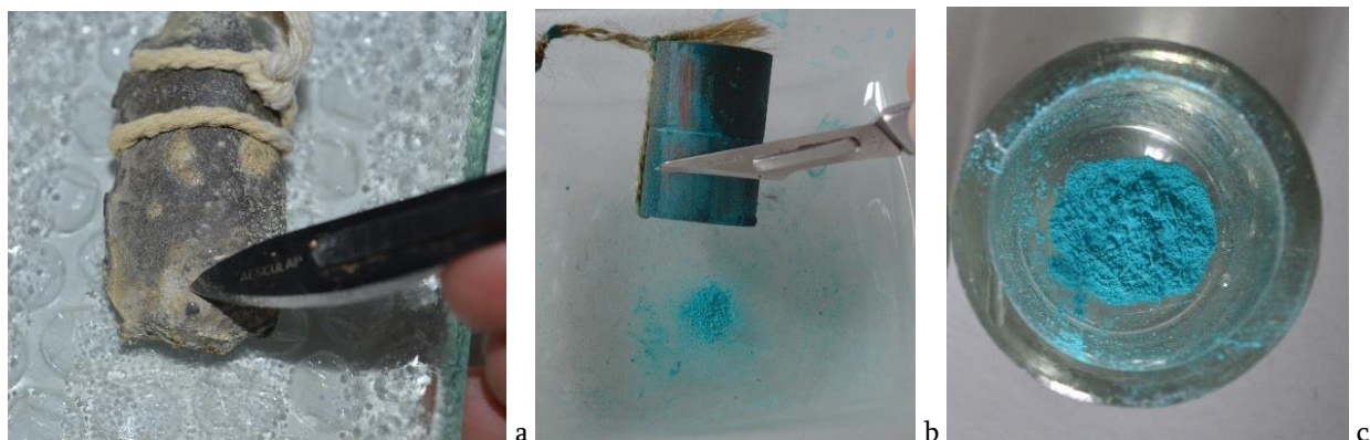
Fig. 10. Aspects from the process of the preparation of (a) lead white and (b)-(c) copper-based pigments. The metals were suspended in bottles with vinegar. The pigment is respectively a white or greenish blue corrosion layer formed on the metals as a result of a complex atmospheric corrosion process. The pigment was removed from time to time and a new corrosion layer then formed. Credits Dumitrița Daniela Filip.
